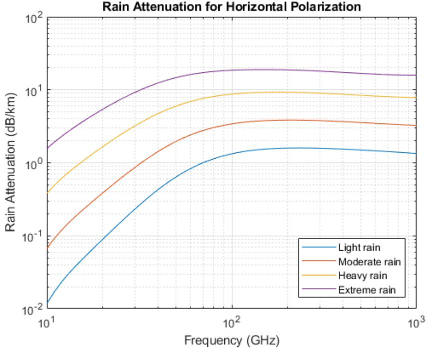
Fig.9.2 - Rain attenuation for different bands and rain strength (logarithmic scale) (replace)
