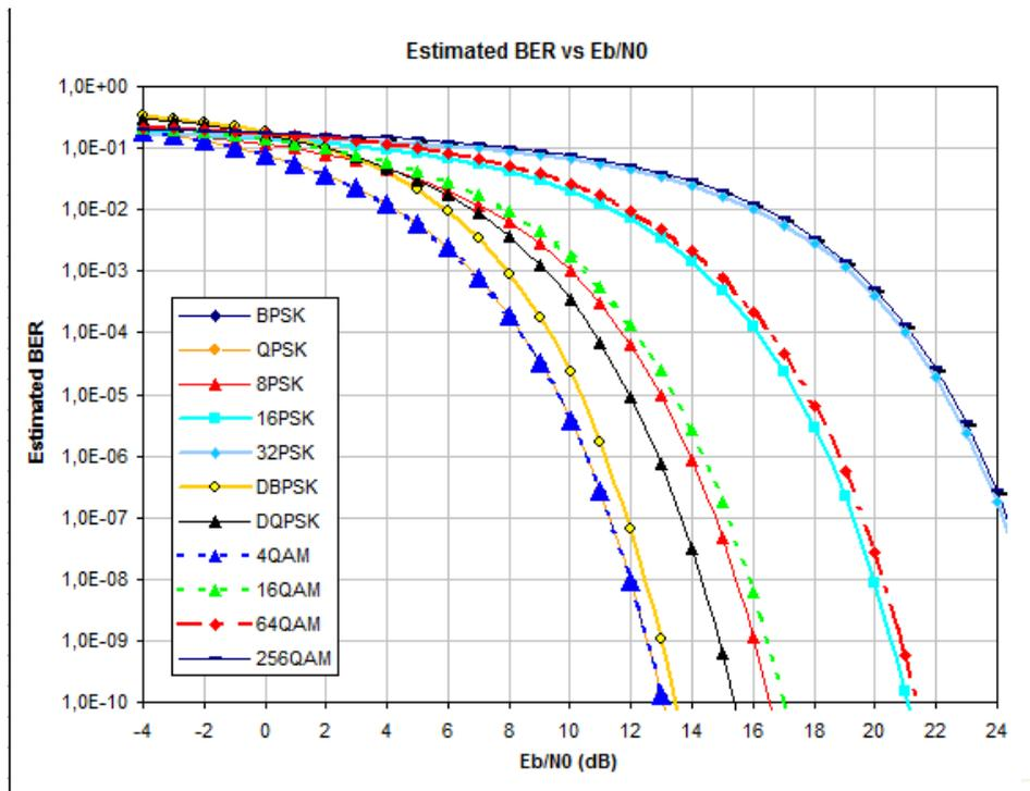
Fig.9.1 - Bit Error Rate as a function of  $E_b/N_0$  in dBs for different modulation schemes.
